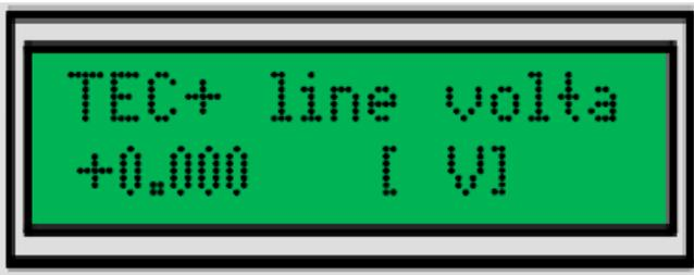
The TEC is powered with negative voltage. This means, the voltage at positive line is close to 0 V (0 ... - 0.5 V).
