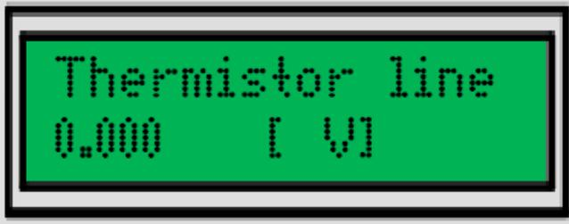
This line is normally at ground potential. However, if the connection to the PTCC is weak, the line is pulled up by the thermistor and line 1, and the value is higher.
