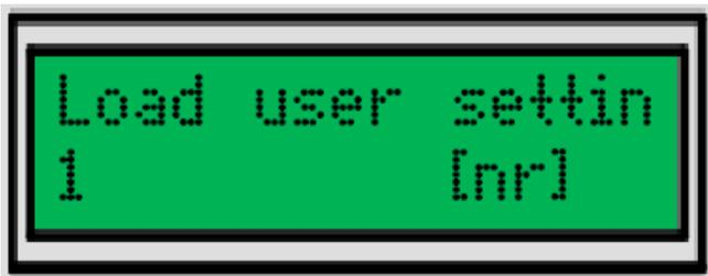
User can load the **PIP-DC** settings from one of four memory banks. Choosing "Load user settings" results in replacing current **PIP-DC** settings with the settings from the bank.
