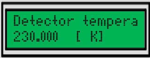
Detector temperature measured by PTTC-01-ADV.
