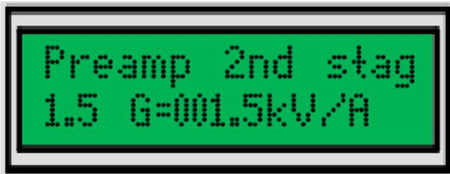
The gain setting is responsible for the gain of the second stage. Please note, than the full output voltage range is available, when the gain is set between 5 V/V to 50 V/V.
