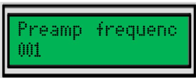
The parameter changes the frequency compensation for the preamplifier first stage. The lower value means the capacitance parallel to the feedback resistor is relatively high, and therefore the circuit might be over-compensated.
