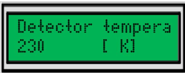
In general, the parameter is responsible for the detector temperature stabilized by the **PTCC** controller.
