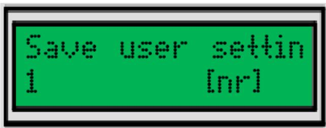
User can store the **PIP-DC** settings in one of four memory banks. When "Save user settings" is chosen, current configuration is saved.
