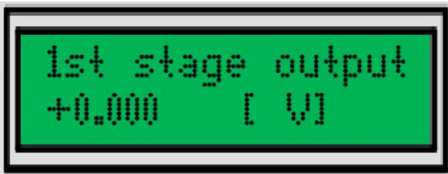
This measurement allows the user to check what is the DC IR radiation level, even when AC coupling to the second stage is chosen. This may be potentially useful in heterodyne detection.
