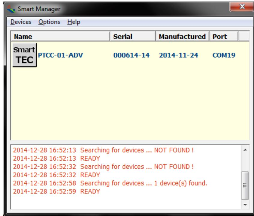
You can see a device list if the list is empty check USB connection and reload device list.
