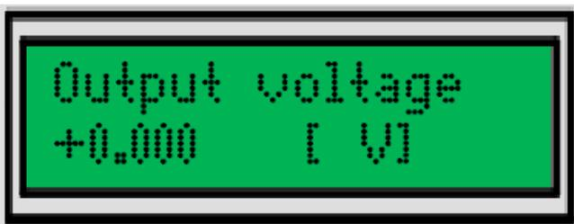
The output voltage measurement is useful especially, if it is not possible to validate the setup connection with the oscilloscope. It is also easy to perform an offset cancellation with no additional equipment.
