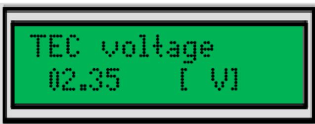
Thermoelectric cooler voltage measured by PTTC-01-ADV.
