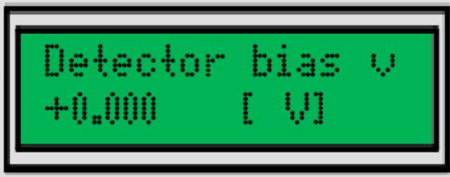
This is the real measured voltage over the detector. This measurement is particularly useful for checking the results of coarse adjustment the detector bias voltage with the digital potentiometer.
