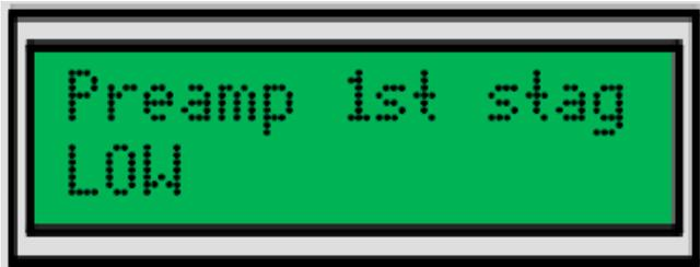
Higher transimpedance results in lower bandwidth (usually around 80 MHz, depending on detector type) and the frequency compensation should be weaker. Preamp is normally more stable and less noisy ( $5 \text{ pA}/\sqrt{\text{Hz}}$  )
