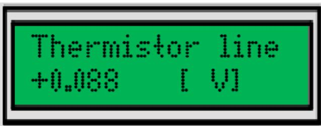
During the normal operation, the voltage here depends on the temperature and should be between 0.5 V and 2 V.
