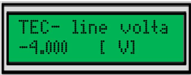
The TEC is powered with negative voltage. This means, voltage at negative line is higher in terms of absolute value, and in normal operation potential is lower than GND (-1 .... -9 V).
