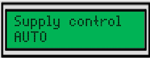
**AUTO** the power supply for the module is turned on, when the valid detector temperature is reached (default)
