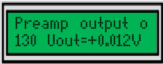
Output voltage 0 V should appear at the output for the potentiometer setting close to the half of the range (128).
